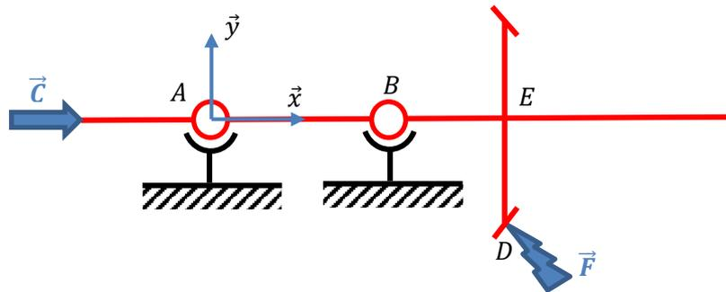
$$AB = a = 106 \text{ mm} - BE = b = 42.59 \text{ mm} - ED = R = 28.6 \text{ mm}$$
